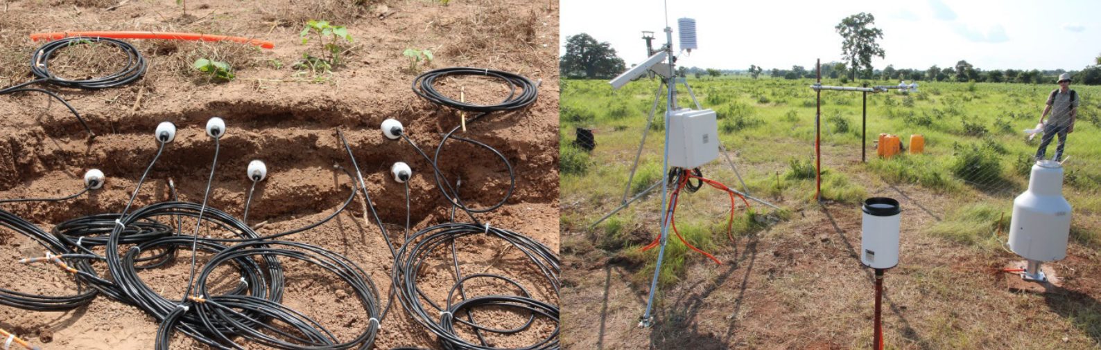
Fig. 1: Soil water sensors of a soil water station (left) and advanced climate station (right) in Dassari. Photograph: Gero Steup 2013.
