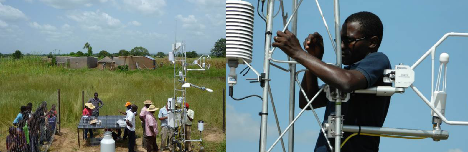
Figure 2: Installation of micro-meteorological stations for investigating the impact of land surface changes on water, energy and CO 2 fluxes in the West African Sudanian Savanna.
